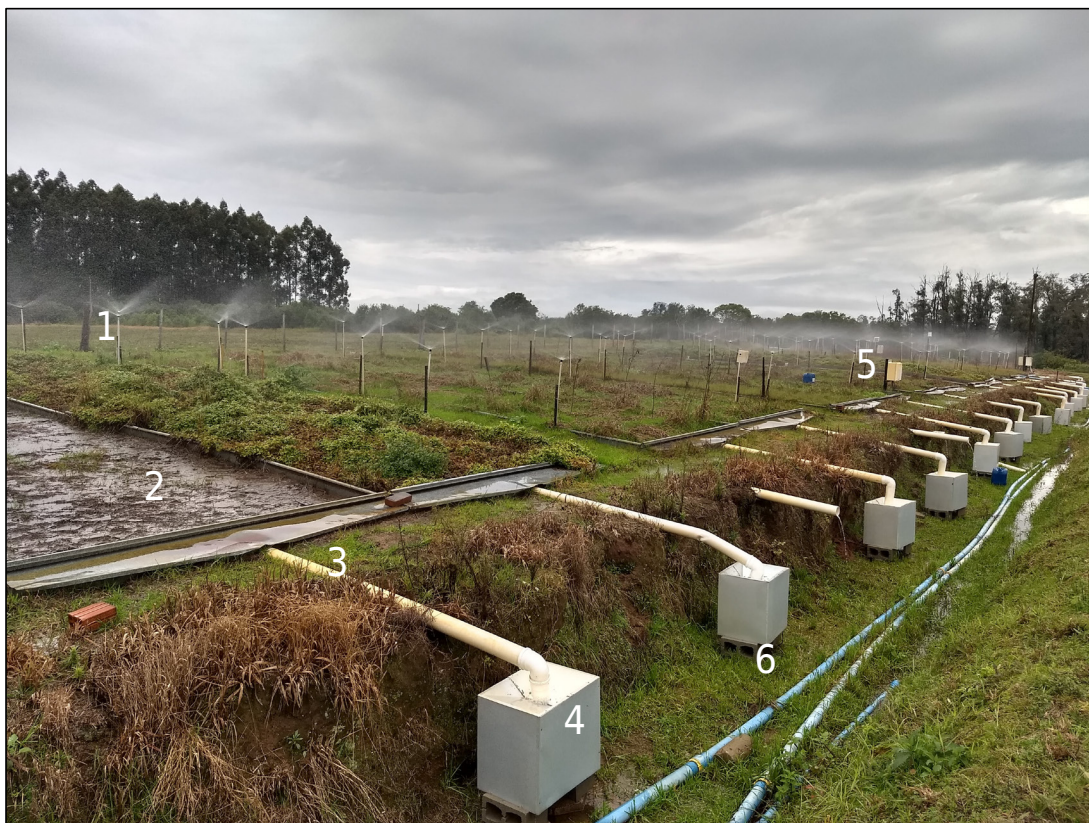
Figure 2. Overview of the experiment at plot scale (14.5 × 3 m) with automatic surface runoff monitoring. 1: sprinklers used for precipitation simulation; 2: experimental plot with exposed soil; 3: PVC pipe for directing surface runoff to the prototype with a tipping bucket system (4), connected to a datalogger (5); 6: concrete base for securing the prototypes.
